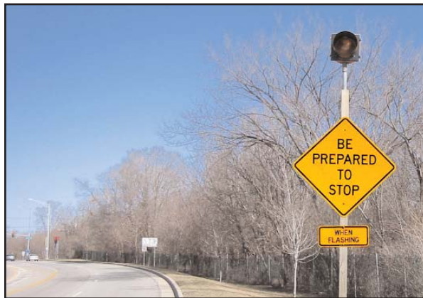
Figure 3–18. Example of AWF and Sign.
